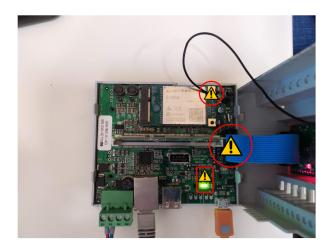
To remove the compute module of the gateway open the metal locking clips of the compute module connector (1) and tilt the compute module towards you (2).
